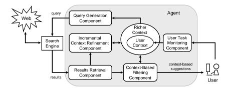
Figure 1: Agent system architecture for incremental context-based Web retrieval
