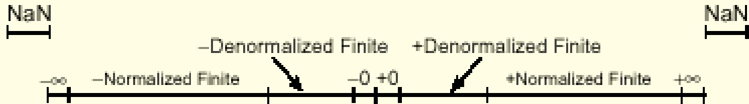
Real Number and NaN Encodings For 32-Bit Floating-Point Format
